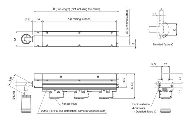
For sizes 1,600 mm (emitting surface) or longer, a cable comes out of each end of the Light Unit.
