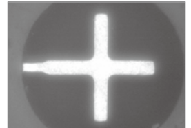
BGA Alignment Mark Inspection
