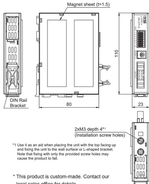
\*1 Use it as an aid when placing the unit with the top facing up and fixing the unit to the wall surface or L-shaped bracket. Note that fixing with only the provided screw holes may cause the product to fall.
