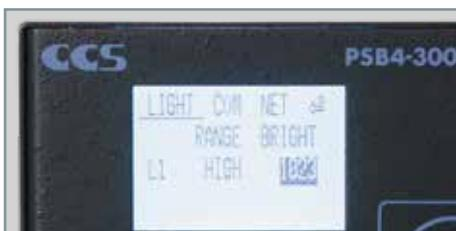
Light intensity levels can be selected only when using manual control and parallel communications. Ethernet communications is fixed to 1,024 levels.
